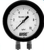
P336 - Series Duplex Pressure Gauge Dial : \varnothing 100 mm Range : 0-4 to 0-35kgf/cm 2 Casing Al, Element 316ss
