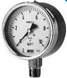
P257 - Series Solid Front Type Pressure Gauge Dial : \varnothing 63, 100 mm Range : -1-0 to 0-1000 bar Casing 304ss, Element 316ss
