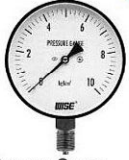
P110 - Series General Service Pressure Gauge \varnothing 40, 50, 60, 75, 100, 150, 200 mm -76cmHg, -76-20 to 0-1000kgf/cm 2 Casing steel, Element Brass
