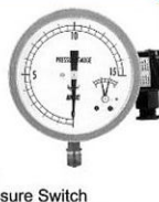
P339 - Series Safety Pattern Pressure Gauge Dial : \varnothing 125 mm -76cmHg-0 to 0-2000kgf/cm 2 Casing Al, Element 316ss
